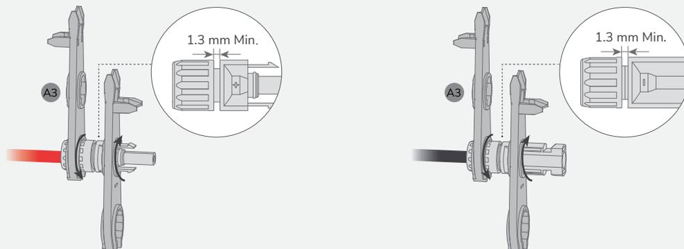
b. Check the polarities of the connection cables.
